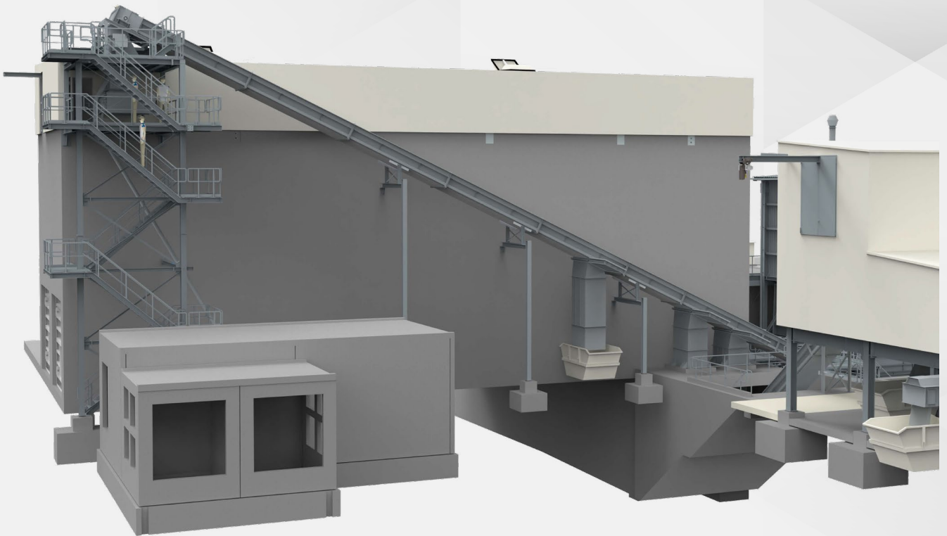
AF (alternative fuel) storing with automatic reclaimer
