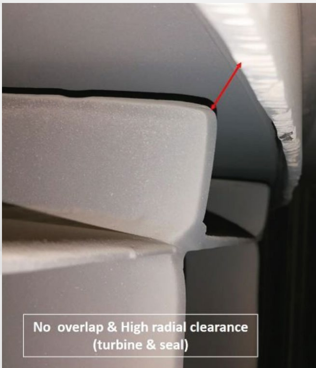
Defected Top seal (pic#1)
