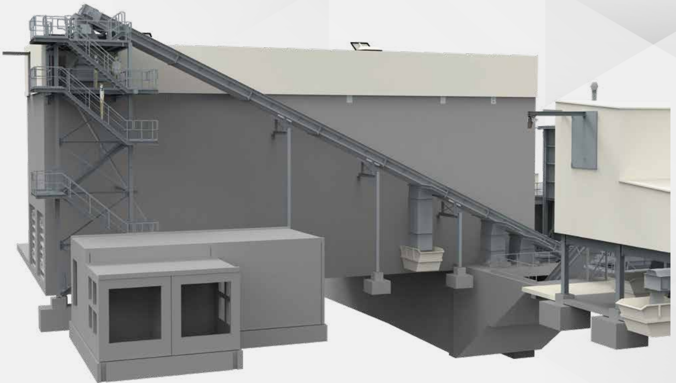
AF (alternative fuel) storing with automatic reclaimer
