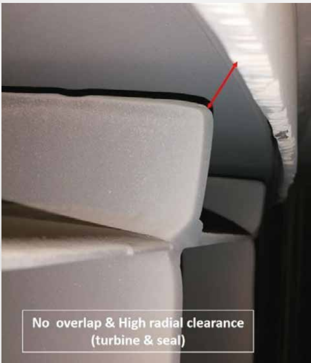
Defected Top seal (pic#1)
