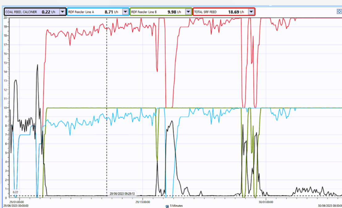
Figure 1. The chart illustrates how the three Pfister feeders act in conjunction with PXP control. The coal is minimised but kicks in when the SRF feeders reach their maximum – and when a SRF feed line blocks. Initially the FUELFLEX is not operated. Then SRF feed to it is ramped up to 10 t/h with SRF line A to the calciner controlling the bottom stage temperature. Each time an SRF line blocks the coal replaces it – and when SRF feed reaches the 20 t/h limit coal feed supplements to control the calciner temperature. Otherwise, the coal is maintained at the 0.2 t/h minimum.
