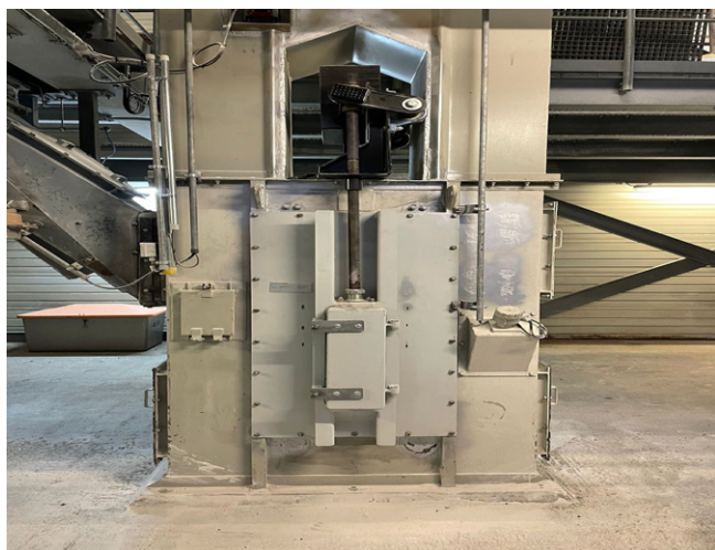
Picture 6: The parallel take-up device ensures that the take-up pulley is limited to parallel movement.
