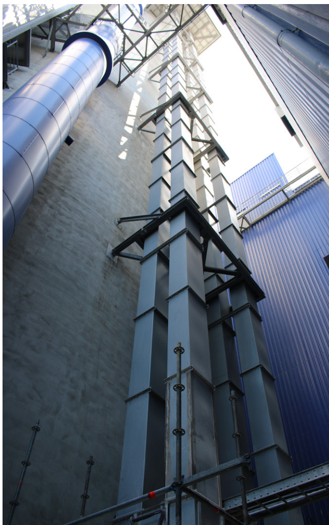
Picture 8: With this modernisation, the cement manufacturer was able to increase the conveying capacity of the bucket elevators for the cement silo feed.
