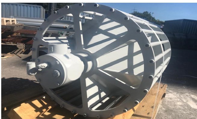
Picture 7: To avoid caking, the take-up pulley is designed as cage-type foot pulley and is provided with a double deflection cone. For this order, the screwed and hardened version of the cage-type foot pulley has been used.
