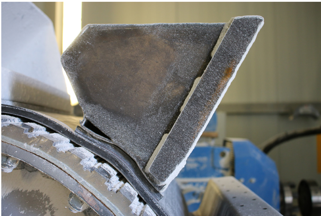
Picture 4: No material can penetrate between belt and bucket.
