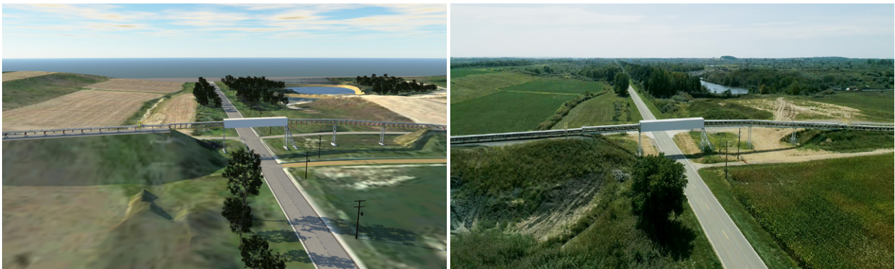
Pictures 4 + 5: on the left: 3D model of the highway crossing during the project planning phase; on the right: real picture after commissioning of the same section
