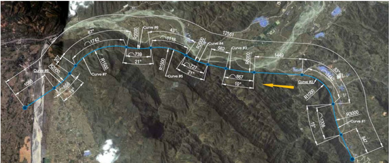
Picture 1: "BEUMER Group implemented an overland conveyor in China that is able to curve on 85 percent of the 12.5 km long conveyor line.
