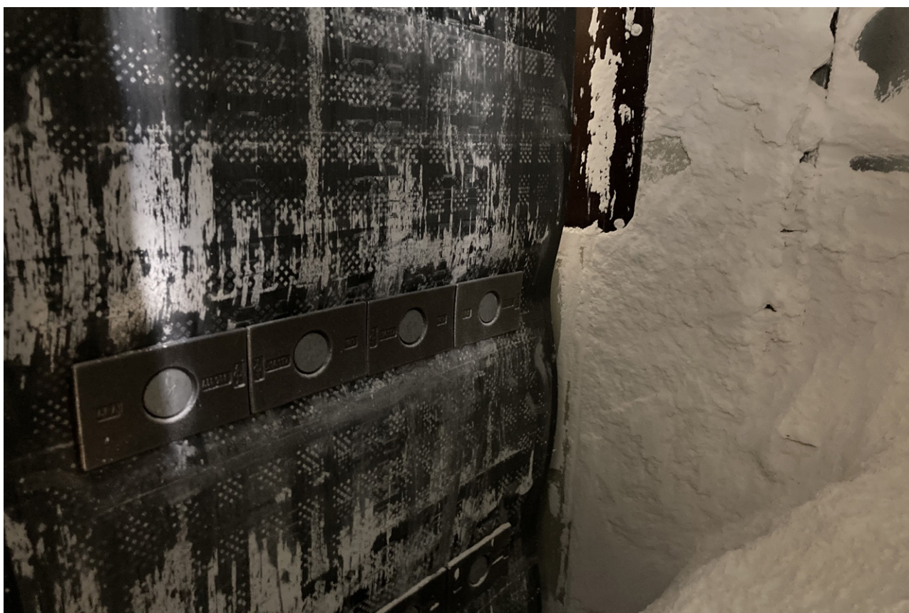
Picture 5: The buckets are mounted with forged segments and screws on the back side of the belt.
