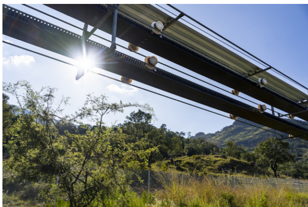
Doppelmayr_BooySendalNorth_06.jpg - The axles are fitted with plastic running wheels which run on fixed anchored track ropes and guide the belt.
