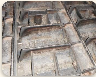
Figure 6: Wear on the ETA cooler lanes over several years
