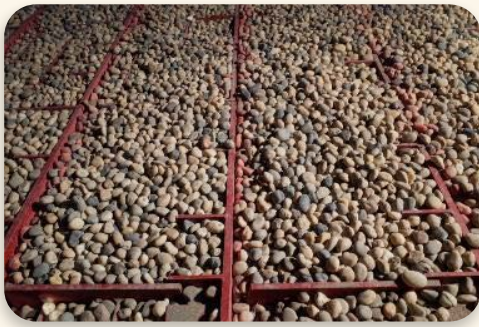
Figure 6: Wear on the ETA cooler lanes over several years
